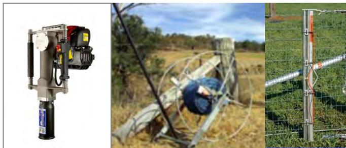
**Fencing**- We also now have a maxi-driver to assist with fencing; this hand held driver weighs around 17 kg and is ideal for driving steels posts, including larger ones. We decided to also purchase a netting strainer large enough for netting up to 1500mm wide and a 3 way wire spinner.
